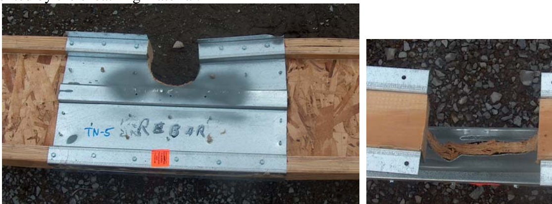
Figure 7: Failure of FlangeGW90 Showing Close-Up of Flange Buckling
