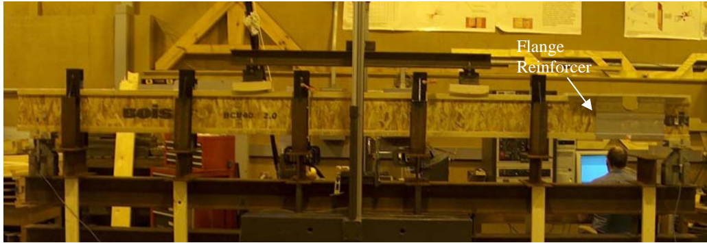
Figure 2: Simply Supported Beam with Load Applied at the Third Points, Specimen With Flange Reinforcer With Sheathing 11" From Support
