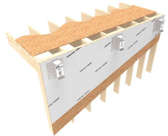
Step 1 – Mount Deck Bracket To Double Blocking
